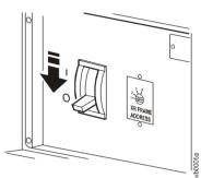
**3** Set the PDU **Main Input** circuit breaker (or switch) to OFF.
